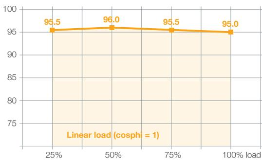
With a transformerless design and Energy Saving Inverter Switching (ESIS) technology, the Kohler PW 6000 delivers high efficiency at partial and full load (up to 96.0% in double conversion online mode). This level of efficiency dramatically reduces the total cost of ownership of the UPS system during its life cycle.
