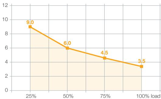
The Kohler PW 6000 actively manages the input current total harmonic distortion (THDi) at a low level (3.5% at 100% load). Kohler PW's unique technology neutralises the emission of harmonics at the input of the UPS system, providing greater reliability of operations for circuit breakers and extending the overall service life of the equipment.
