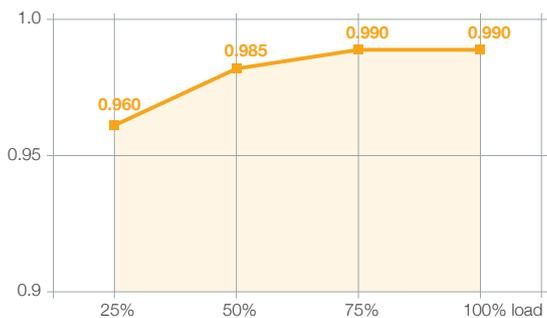
Thanks to the near-to-unity input power factor of 0.99, the Kohler PW 6000 reduces the input installation costs by enabling the use of smaller cables. Furthermore, it avoids the unnecessary use of additional phase compensating devices, which consequently keeps the overall UPS efficiency high.
