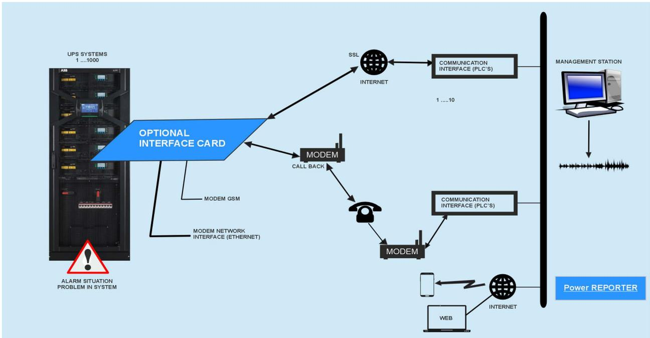
PowerREPORTER™ is a remote monitoring and management service which is a part of the premium power protection concept. Two solution cards are available to enable connection between the UPS and the outside world: 'Modem/Ethernet' or 'Modem/GSM'.
