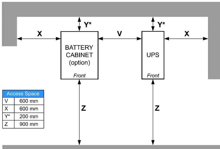
The above diagram illustrates the recommended clearances to be provided around the UPS and optional Battery Cabinet. Please read the following notes for clarification.
