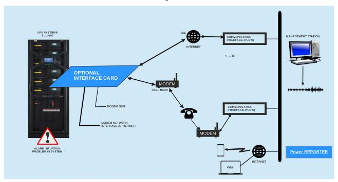
PowerREPORTER™ is a remote monitoring and management service which is a part of the premium power protection concept. Two solution cards are available to enable connection between the UPS and the outside world: 'Modem/ Ethernet' or 'Modem/GSM'.
