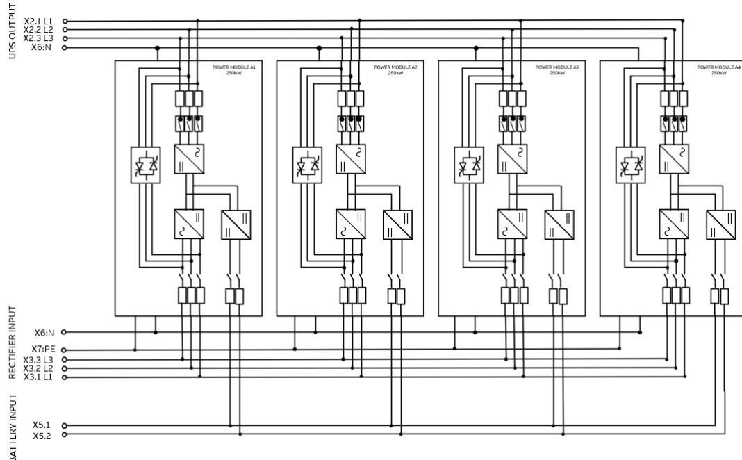
**Note: The above Schematic shows a 1000 kW Frame. If a 1500 kW Frame is selected, the schematic would have an additional 2 modules**
