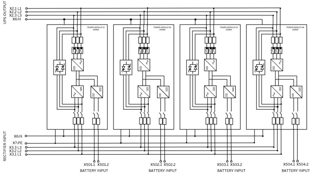
**Note: The above Schematic shows are 1000kW Frame. If a 1500kW Frame is selected, the schematic would have an additional 2 power modules.**
