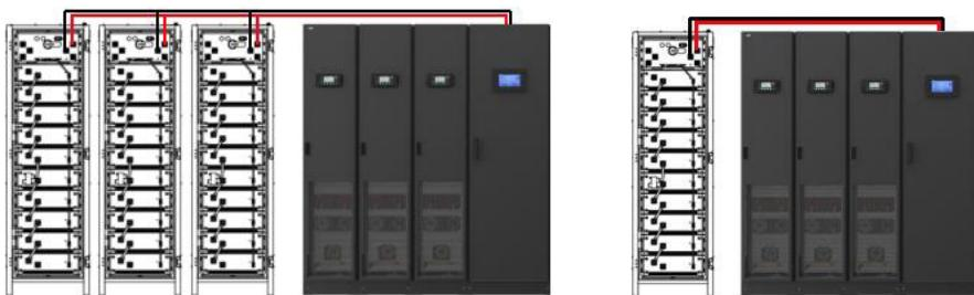
Note: Dedicated per-frame-size Optional - Common Battery connection kit should be added on the MF Series UPS cabinet.
