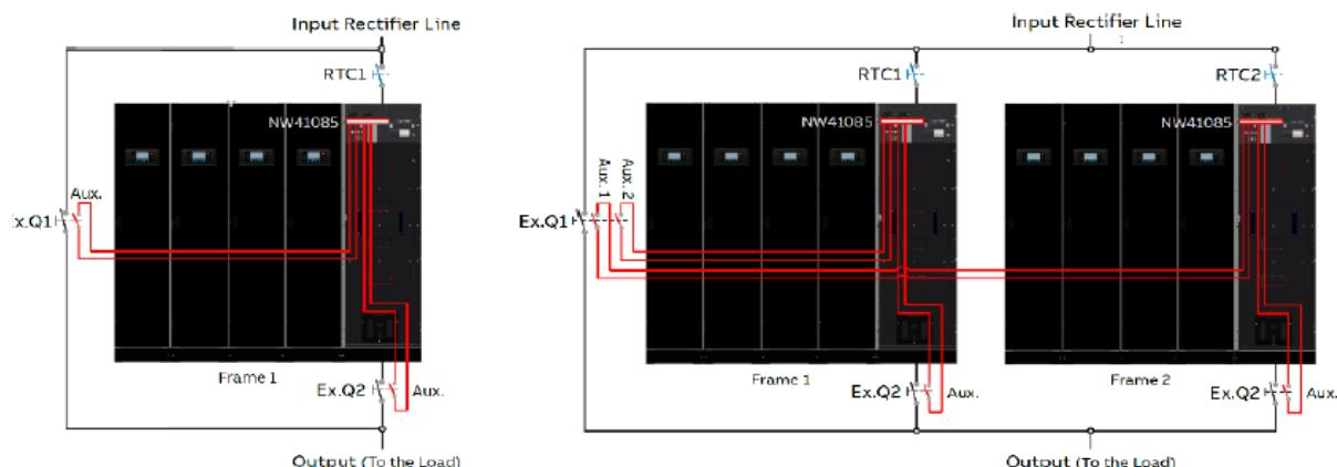
Therefore, the auxiliary contacts of EXT Q1 and EXT Q2 should be connected to the to the input dry port X1 in the communication interface. For more information on the procedure and configuration, refer to the User Manual.
