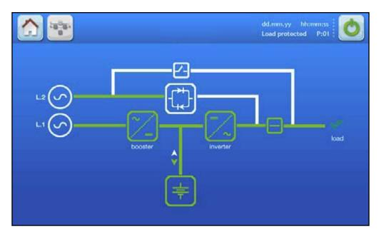
Three meters are included on the mimic display screen to indicate the rectifier, inverter, bypass and load operating parameters. The meter source is selected by touching the associated power block on the mimic display. The battery temperature and remaining autonomy time are also displayed.
