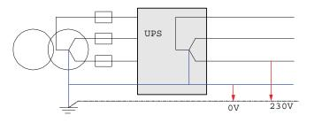
**Key Point:** As the input neutral must be unswitched and connected to the UPS at all times, a 4-pole input switch or isolator must not be used at the LV switchboard on a TN-S system.
