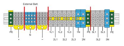
Figure 1 Terminal block connections
