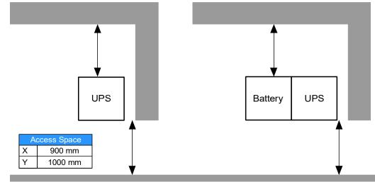
The PW8000DPA RI UPS sub-rack requires rear access in order to connect the power cables, and we recommend a minimum of 900 mm clearance is provided at the rear of the rack cabinet. A minimum clearance of 1000 mm is required at the front of the rack cabinet to allow the UPS assemblies to be installed and serviced.
